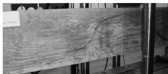
(a) Beam B18-0a (regular concrete and no stirrups)
